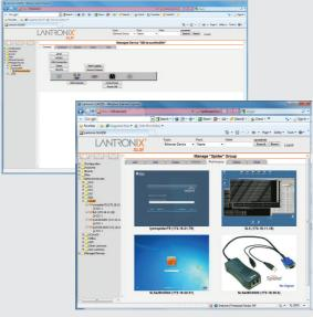
The vSLM integrates various managed device interfaces (console port, power outlet, KVM port) into a consolidated view for simplified access and control of your servers and IT infrastructure equipment.
